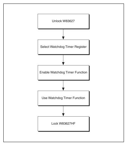
Figure C-1. Watchdog Timer Programming Procedure
